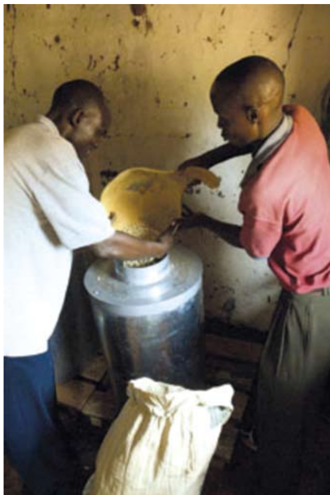
This hermetic metal silo protects harvests from pests.
